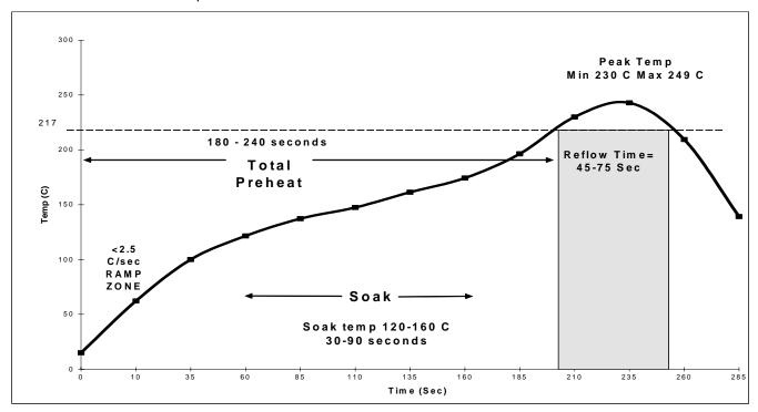
**Ramp Zone**- the ramp zone is used to elevate the temperature of the PCB to the desired soak temperature. In the ramp zone the temperature of the PCB is constantly rising, at a rate that should not exceed 2.5 C/sec. The oven's ramp zone should normally occupy 25-33% of the total heated tunnel length.
