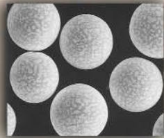
Sn63 Solder Powder 600X By SEM
